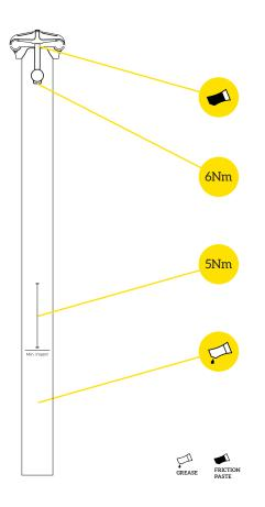
Your new carbon seatpost withstands highest stress and has been made to the latest and most efficient methods of design and manufacture. This includes special features that must be considered for installation.
